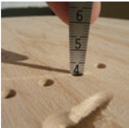
Taper gauge is easy to check the hole diameter.
