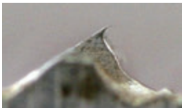
Enlarged CP files tooth. This tooth shape is the secret of why CP file works fine!
