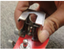
10mm Hex Nut Gotoh® or other guitar tuner hex nut etc. Use GNC after loosening strings or remove strings.
