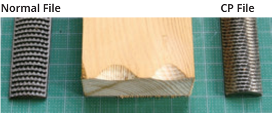
Comparison between CP file and normal wood file Left : 10 strokes by normal wood file Right : 1 stroke by CP file
