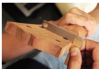
Checking flatness for installing machine heads
