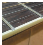
The edge is very sharp after sanding by beveling file.
