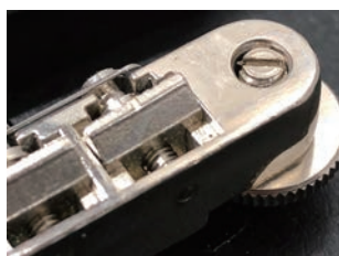
Good to make notches for strings on the metal saddles.
