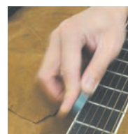
Sanding the fret edge by FSR150 softly.
